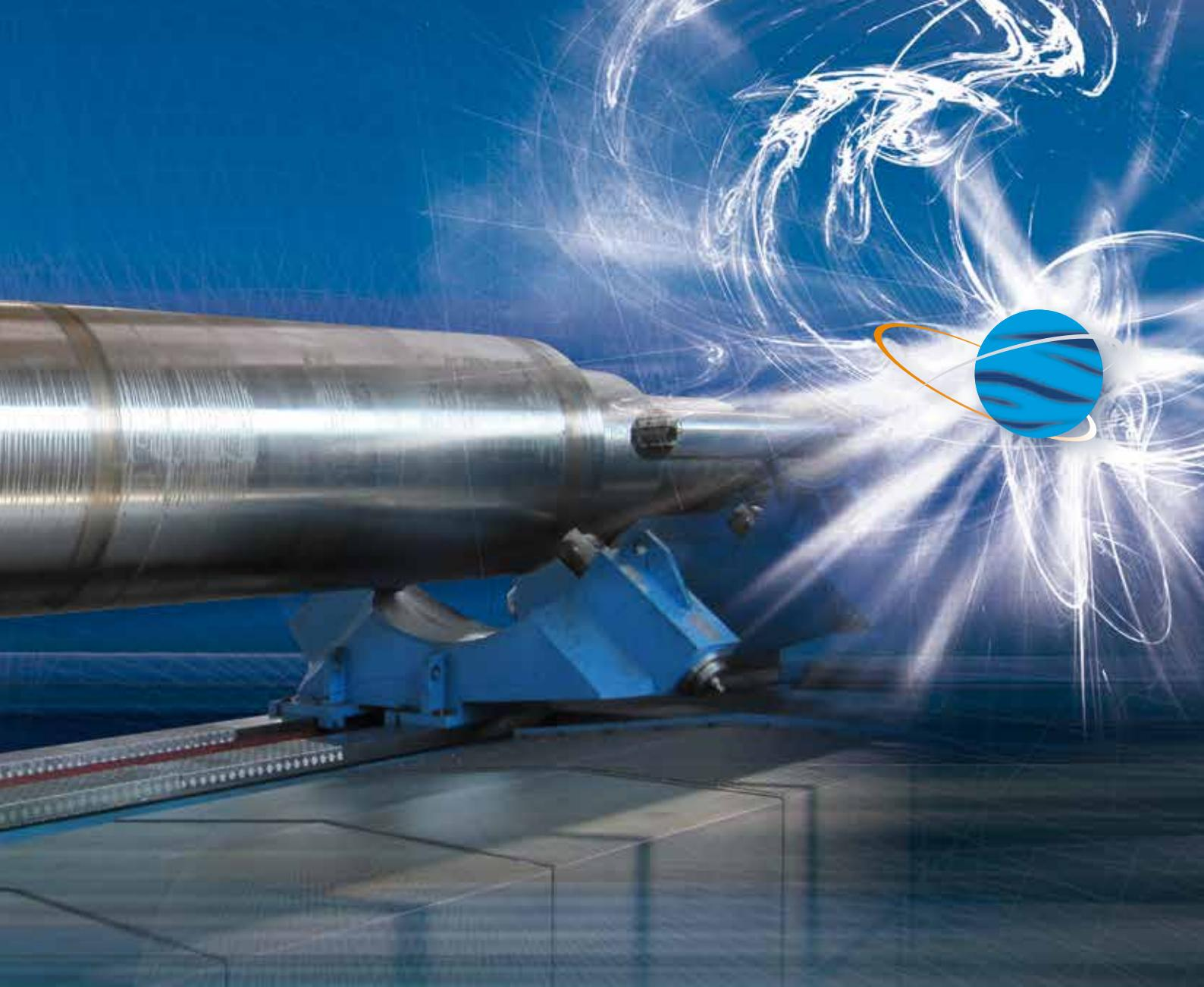
The headstock is configured to house all the drive system components that transmit power to the spindle by means of a series of over dimensioned gears that leverage all the available torque. The spindle in steel forged with cemented, tempered and ground NiCrMo is supported by TIMKEN conical roller bearings with adjustable clearance. The head is lubricated by means of a forced and controlled lubrication system, which is specifically designed to control thermal elongation.
