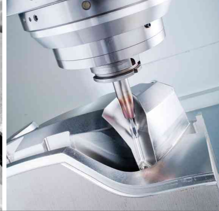
5-axis with R0.5mm pencil cleaning
