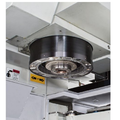
High speed (Fanuc / α22 / 7000i) with gearbox (1:4)
