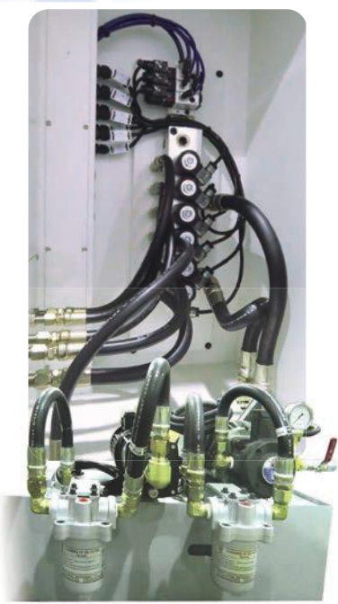
High pressure Coolant High pressure with 25 Bar with filter
