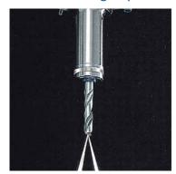
Tool breakage detector
