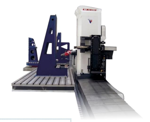
A Floor type horizontal boring mill WF type is designed for precise and highly efficient coordinate boring, drilling, milling, and cutting of threads of big and heavy work pieces up from cast iron, cast steel and steel. The machine can be equipped with floor plates and/or rotary table(s) according to machining requirements. As with all Fermat Boring Mills a wide range of accessories can be added that considerably enhance the machine's versatility.
