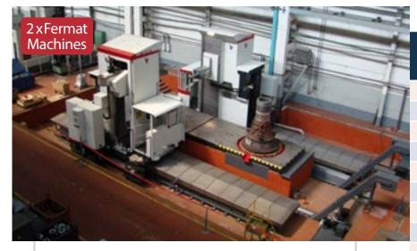
OTHER FERMAT MACHINES WFT 13 R CNC, APC | X=2 000 mm | Y=2 000 mm | Z=1 500 mm | W=730 mm Rotary Table 1 600x1 800 mm | CTS 50 bar | ATC 60 | D'Andrea UT 5/5000S
