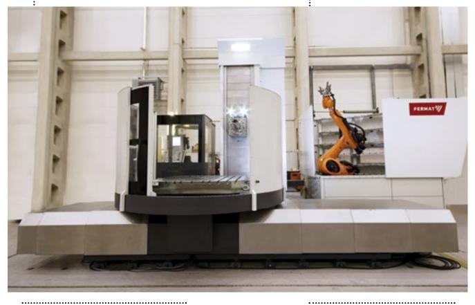
Robotic Tool Changer - Max. Capacity 210 tools
