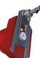
Automatic Facing Head FH 65/80 Plate Diameter: 650/800 mm | 19.68"/31.50" Positioning: Automatic Boring Accuracy: 0,05 mm | 0.002" Radial Traverse: 170/220 mm | 6.69"/8.66" Maximum Boring Diameter: 1200/1400 mm | 47.24"/55.19" Coolant Through Spindle: Not Possible
