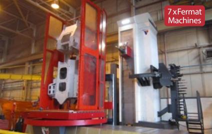
OTHER FERMAT MACHINES WFT 13 R CNC | X=3 000 mm | Y=3 500 mm | Z=1 500 mm | W=730 mm | Rotary Table 2 000 x 2 400 mm | CTS 20 bar | ATC 60 WFC 10 CNC | X=2 000 mm | Y=1 700 mm | Z=1 250 mm | W=730 mm | Rotary Table 1 250 x 1 400 mm | CTS 20 bar | ATC 20
