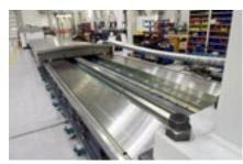
X-Axis Hydrostatic guideways
