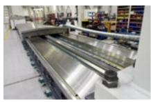
X-Axis Hydrostatic guideways
