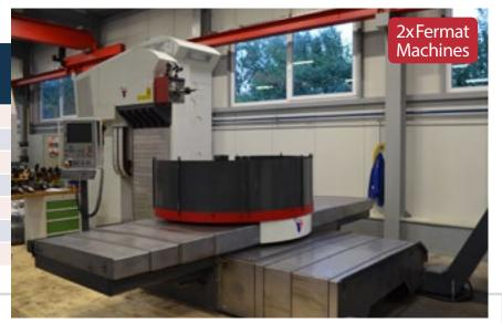
OTHER FERMAT MACHINES WFT 13 CNC (2pcs) | X=4 000 mm | Y=2 500 mm | Z=1 700 mm | W=730 mm | Rotary Table 1 800x2 200 mm | CTS 20 bar, ATC 32, UHM, Angular Clamping Plate 800x1000x2150, 2 servomotors
