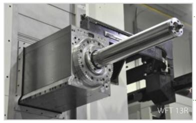
due to the spindle axial force of 40,000 Nm. In WRF and WRFT series, two Y-axis ball screws with two scales control slide ram deflections. The third ballscrew in the torque position that is constantly pushing the headstock body upwards is added for 150 and 160 mm | 5.91" and 6.30" headstock. The upper part features heavy duty INA roller linear guideways, further contributing to the precision and rigidity of the machine.
