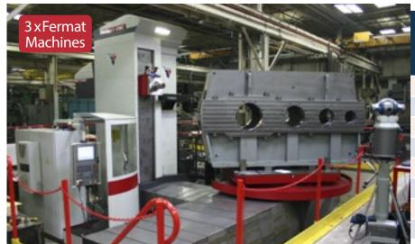
OTHER FERMAT MACHINES WFT 13 L CNC HIGHSPEED | X=2 500 mm | Y=2 000 mm | Z=1 500 mm | W=730 mm | Rotary Table 1 600x1 800 mm | CTS 20 bar | ATC 40, BUC E 85/4000 CNC
