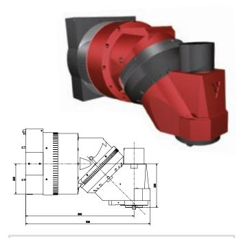
Speed: 10 - 3 000 rpm Power: 30 kW (40 HP) Torque: 1 600 Nm Indexing: 0,001° / 0,001° Clamping torque: A-Axis 3 800 Nm, C-Axis 6 500 Nm
