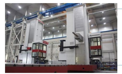
Heavy duty execution of floor type boring mill with ram stroke 1 500 mm (59.06"), 1 000 mm (39.37") spindle stroke with 160 mm (6.30") spindle diameter represents the newest technology and concept of floor-type horizontal boring mills that are currently on the global marketplace. The powerful closed designed headstock consists of a movable slide ram (Z-Axis) and a movable live spindle (W-Axis).
